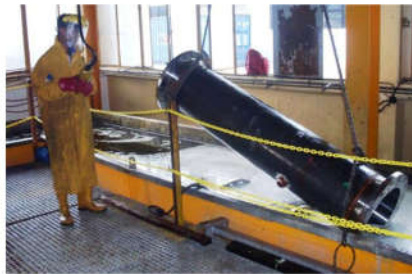
CHEMICAL CLEANING WASH
